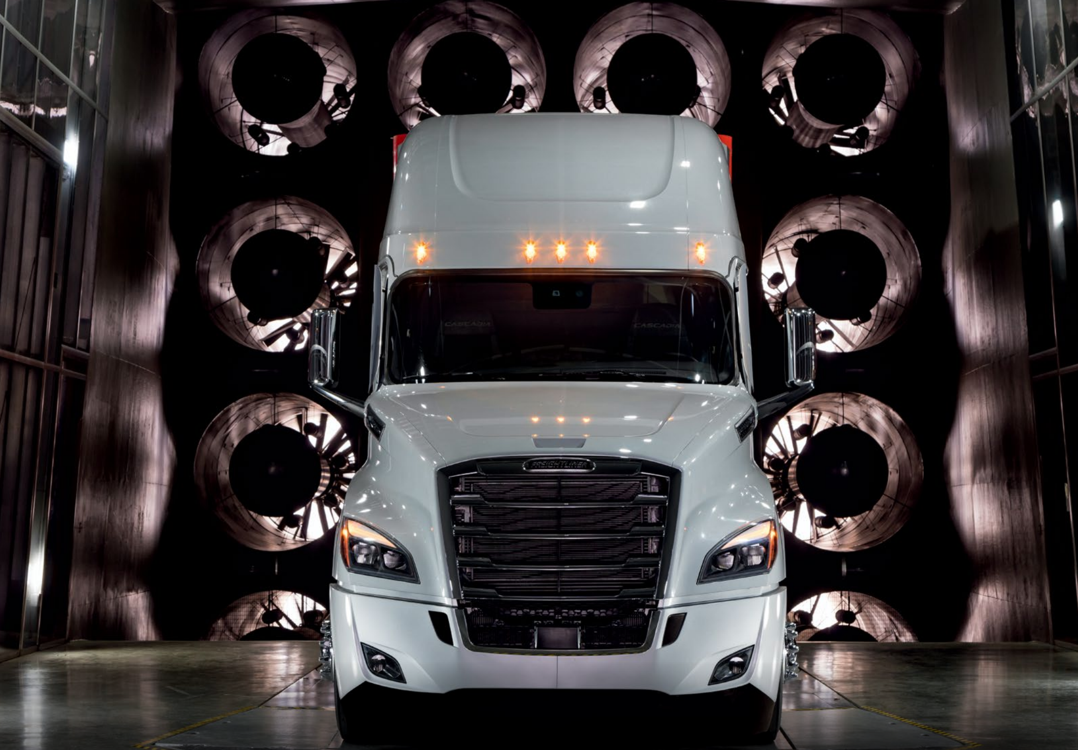
126" BBC 72" RAISED ROOF SLEEPER CAB UNDERGOING AERODYNAMIC TESTING IN DTNA'S PROPRIETARY WIND TUNNEL
