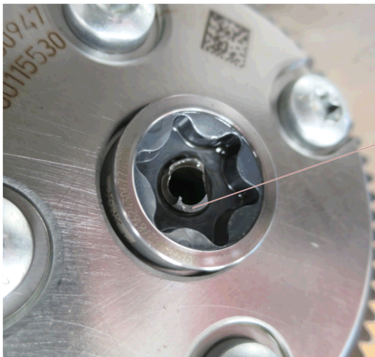
1. Broken Central Valve on Exhaust Camshaft
