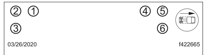
Fig. 4, Axial Bolt Tightening Pattern
