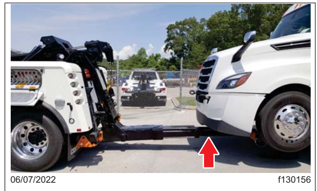
Fig. 23.15, Retracting the Recovery Boom
