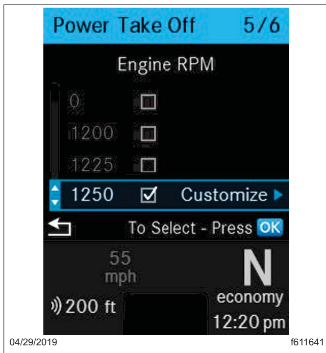
Fig. 3.20, Quick Access Screen: Power Take Off (PTO)
