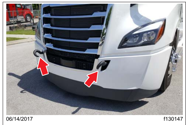
Fig. 23.7, Tow Hooks Installed, Facing Down
