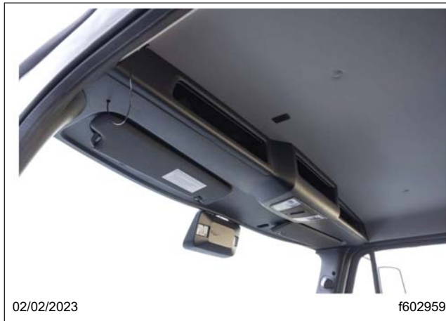
Fig. 3.46, Overhead Instrument Panel
