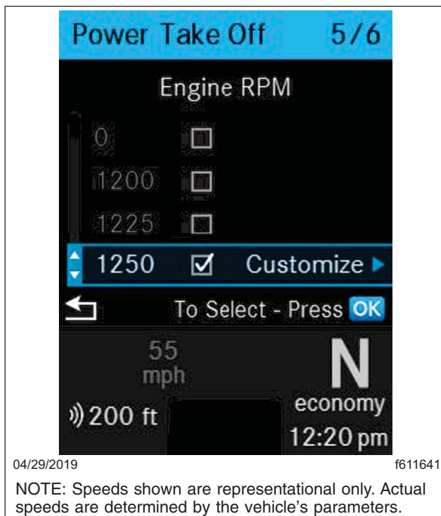
Fig. 10.7, Quick Access Screen: Power Take Off (PTO)
