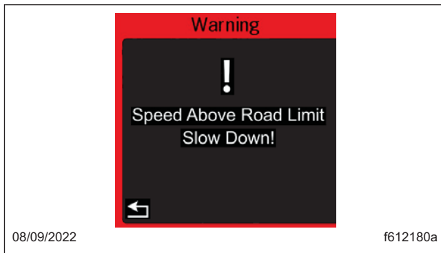
Fig. 6.26, Traffic Sign Display Warning
