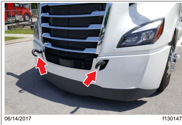
Fig. 13.3, Tow Hooks Installed, Facing Down
