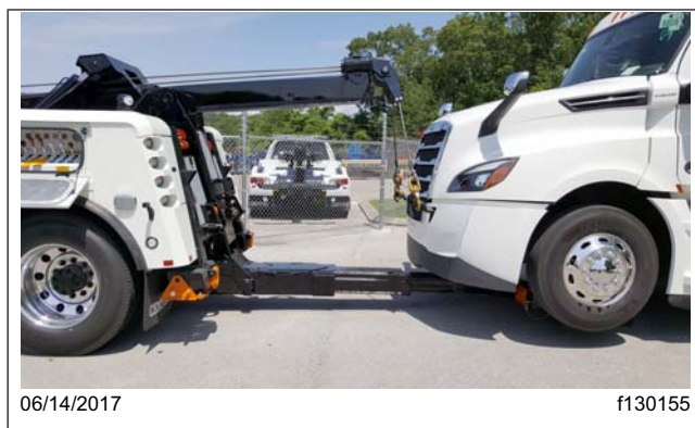
Fig. 13.11, Stinger with Lift Adaptors Under the Axle (tow truck shown)
