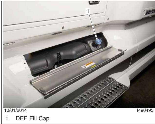
Fig. 12.7, DEF Tank Location (Western Star 5700 shown)
