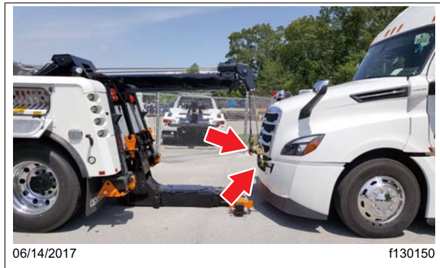
Fig. 24.10, Tow Cables Connected to the Tow Hooks
