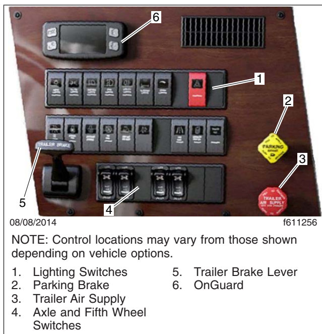
Fig. 4.1, Dash Control Panel
