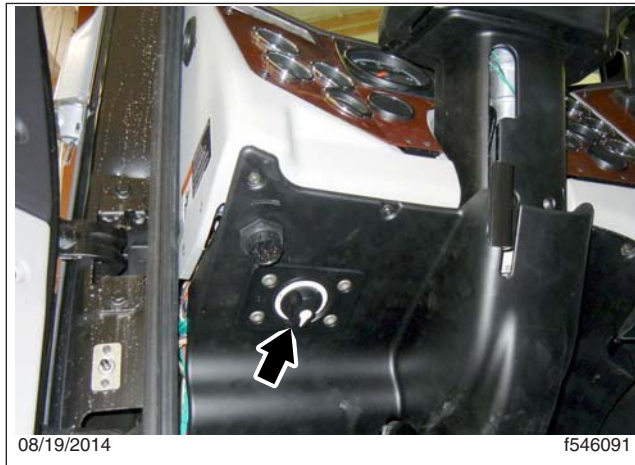
Fig. 9.4, Cab Load Disconnect Switch
