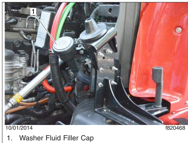
Fig. 23.10, Windshield Washer Reservoir (Western Star 5700 shown)
