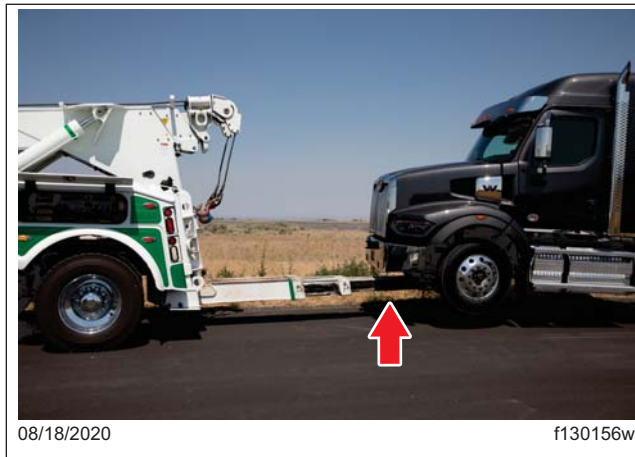
Fig. 24.9, Retracting the Recovery Boom
