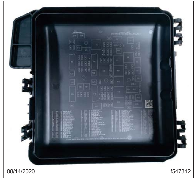
Fig. 9.7, VPDM Inside Cover Map of Fuses and Relays
