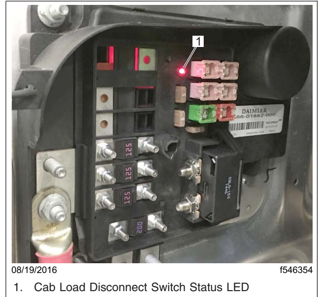
Fig. 9.10, Battery Cable Access Box (engine side)
