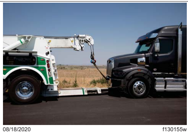
Fig. 24.8, Stinger with Lift Adaptors Under the Axle
