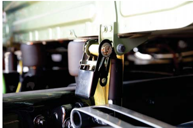
Fig. 24.12, Tension Strap Installed to Hold Down the Cab
