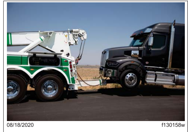
Fig. 24.11, Safety Chains Connected on the Towed Vehicle
