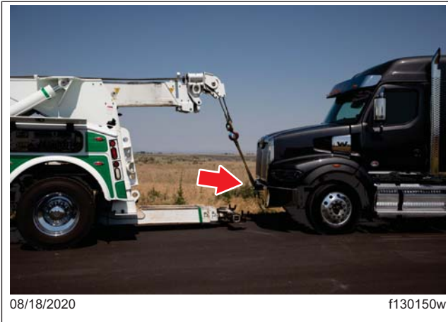
Fig. 24.5, Tow Cables Connected to the Tow Pin
