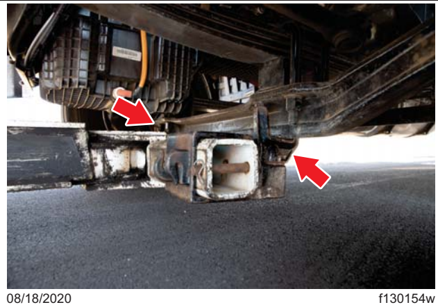
Fig. 24.7, Positioning the Stinger with Lift Adaptors Under the Axle
