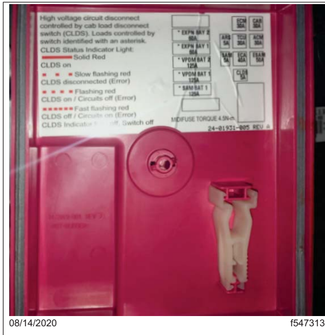
Fig. 9.6, Example Fuse Labeling on BCA Cover
