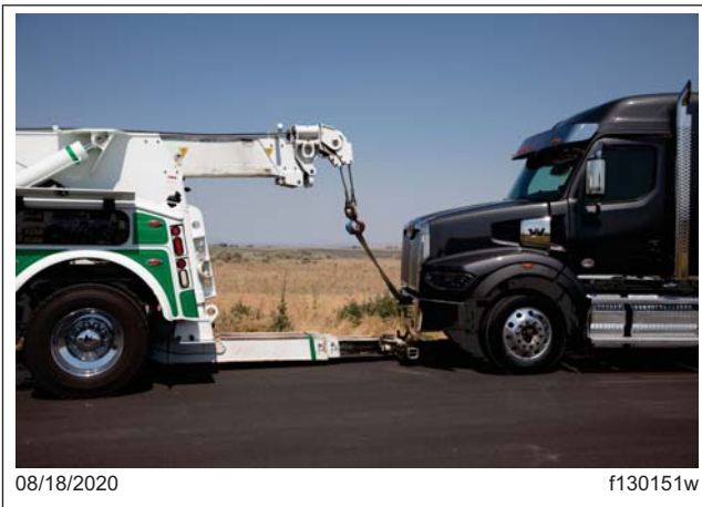
Fig. 24.6, Moving the Stinger and Crossbar Under the Bumper
