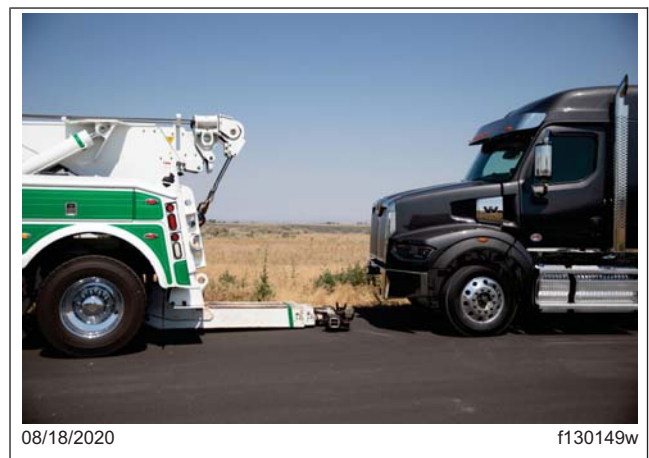
Fig. 24.4, Positioning the Stinger Assembly
