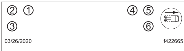
Fig. 10, Axial Bolt Tightening Pattern
