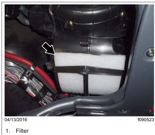
Fig. 4, Cab Recirculation Air Filter
