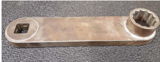
Torque Compensation with Meritor Extension Tool 3256B1354
