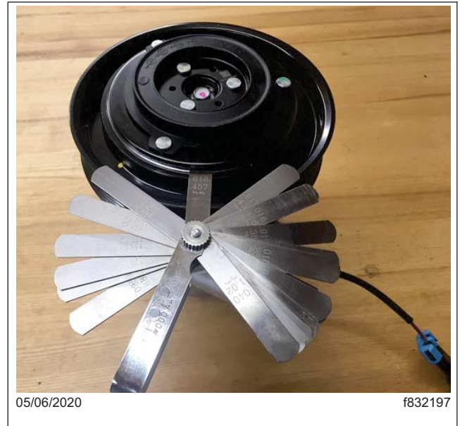
Fig. 1, Valeo Drive Plate Clutch Air Gap
