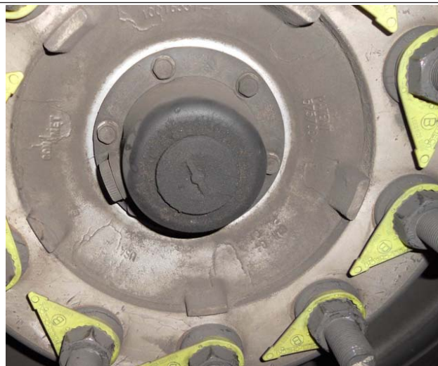
Fig. 14, Normal Oil Venting
